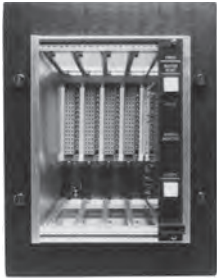
Rear view of Chassis showing Buss Board
